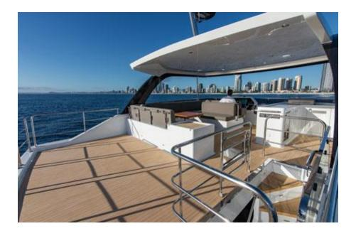
A high bridge deck results in a high freeboard, benefitting not only the internal spaces of the hulls but also the deck space. Even with the voluminous interior on the main deck, the side decks are surprisingly expansive at 650mm. Solid railings run all the way forward, wrap around the bow pulpit seat and continue across the foredeck to the other side. At 750mm high, it creates a safer environment at sea and could be easily secured further for young or furry crew members.
